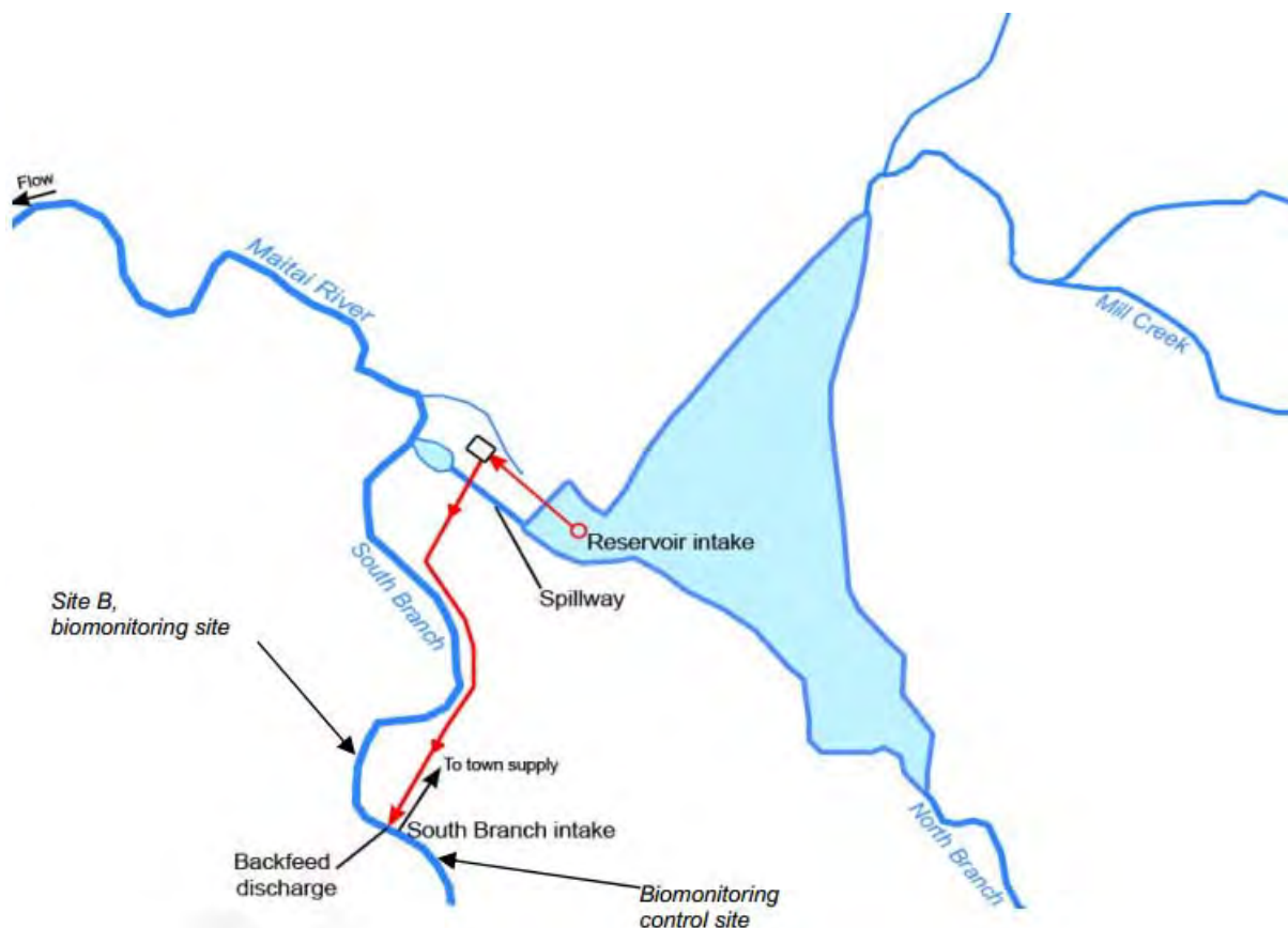
Figure 5. Diagram of the Maitai Water Supply Scheme showing the water supply intake (labelled 'South Branch intake') and back-feed discharge. Also shown are the locations of the bi-annual biomonitoring sites (Holmes 2012). Not to scale.
