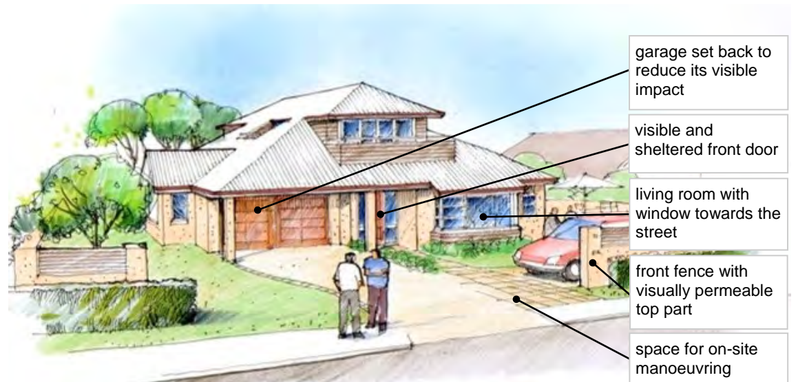
FIG 13: Hand drawn examples of how the rules work out
