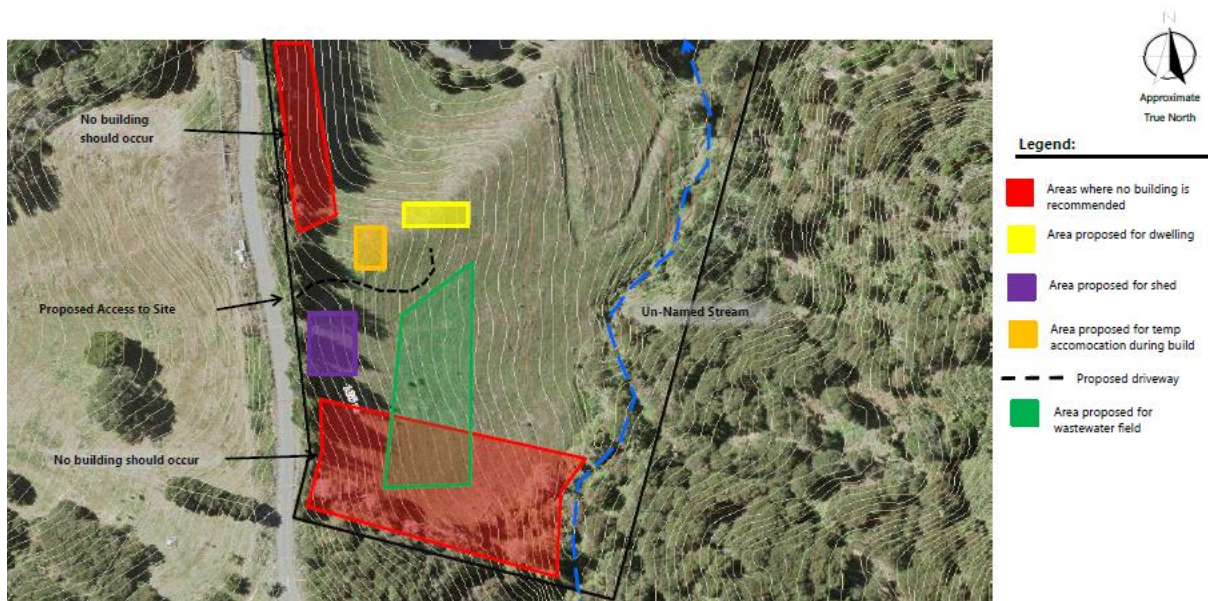
Figure 3: Proposed Conceptual Site Plan (source: CGW drawing 18360/03); note: the RFI response from FEL proposes a different wastewater field location than shown here
