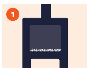
1 Leave a thin bed of ash in the bottom of the firebox
