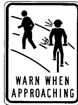
Figure 3: "Warn When Approaching" signs encourage path users to call out or ring their bells (Size 250 W x 330 H)
