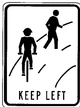
Figure 2: "Keep Left" signs encourage all path users to travel on the left (Size 250 W x 330 H)
