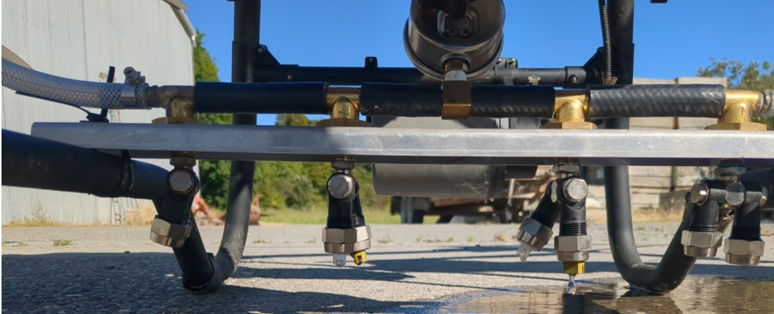
Built bespoke manifold to hold nozzles
